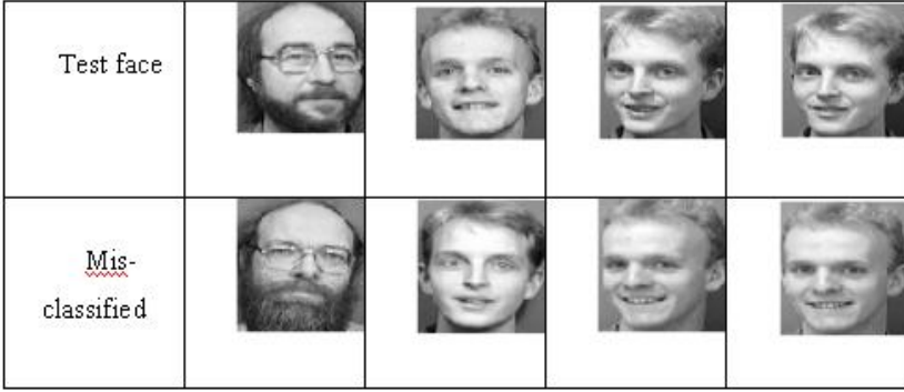
Fig. 2. Mis-classified faces of the 5/5 test (4 errors, 98% accuracy)
